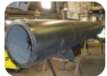
Process vessel required rebuilding and resurfacing. Internal substrates were mechanically abraded and relined using 202 Ceramic Repair Fluid
