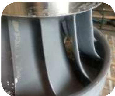
Pump impeller coated with 1mm of 209 EIP PU
