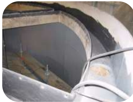
Chemical powder process vessel and chute were lined with 3mm of 209 EIP PU.
