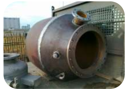
Process vessel operating at 95°C relined using 2 coats of 205 Ceramic HT
