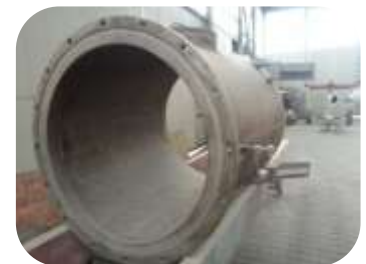
Process vessel required rebuilding and resurfacing. Internal substrates were mechanically abraded and relined using 202 Ceramic Repair Fluid
