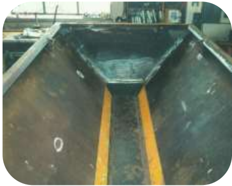
Aggregate sieve abrasive blast cleaned and relined with 3 coats of 209 EIP PU
