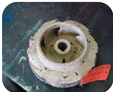
Impeller from a sea water pump was badly eroded. The pump was obsolete and no spare parts were available. The surface of the impeller was rebuilt using 301 Epoxy Resin with glass fillers and then machined to a smooth finish. Once cured 2 coats of 202 Ceramic Repair Fluid were applied to complete the repair
