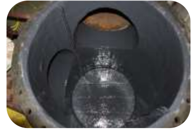
Sea water filter was in need of urgent repair. The internal surfaces were abrasive blast cleaned and lined with 2 coats of 202 Ceramic Repair Fluid. The coating was then post cured at 50C for 6 hrs to ensure the filter was back in operation within 24 hrs.
