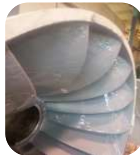
Pump impeller coated with 1mm of 209 EIP PU
